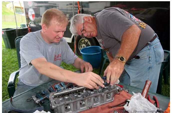
Dave Toler helps Rob Bax rebuild his valve train
